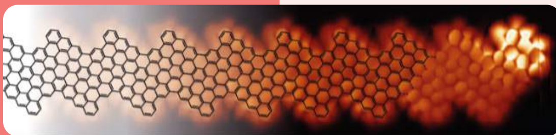
STM image resolving the hexagonal structure (schematically indicated by black lines) of one of the studied GNRs. The bright, localized feature at the right side reveals the emergent “exotic” state at the end of the ribbon.
