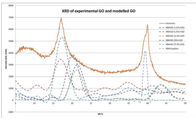
Figure 1. XRD Experimental and simulated patterns of graphite oxide.
