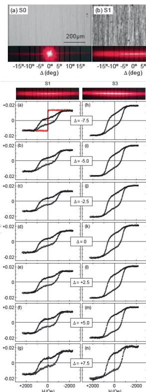
**Figure 1.** Light microscopy images of the different samples employed in this study. For the sake of roughness comparison, all sample stripes are aligned vertically. The scale shown in (a) applies to all pictures. Below the images, we show the scattered laser spots corresponding to each of the samples.  $\Delta$  accounts for the difference in between incidence and scattering angles ( $\Delta = 0$  for specular reflection).
